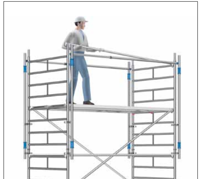
Fig. 6: Safe assembly of rear guardrails using advance guardrail system
